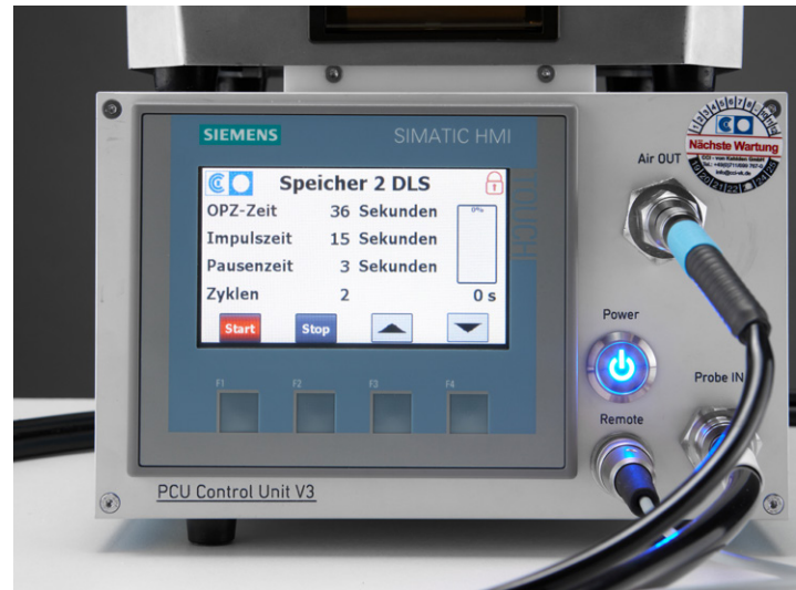
Monitor des Steuergeräts. 4 Programme konfigurierbar // Monitor of the steering unit. It is possible to configure 4 programs
